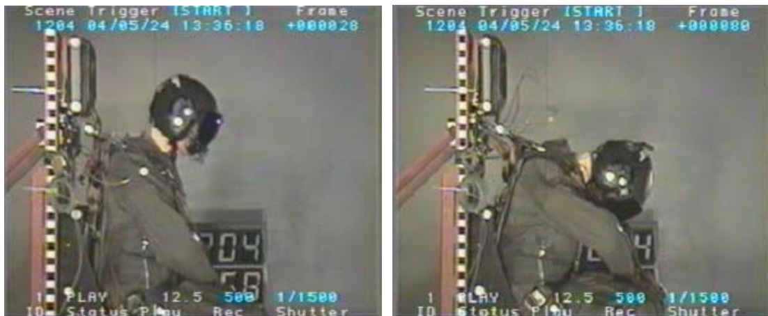
Figure 6: Demonstrating how the markers can disappear into the manikin's shoulder during the test
