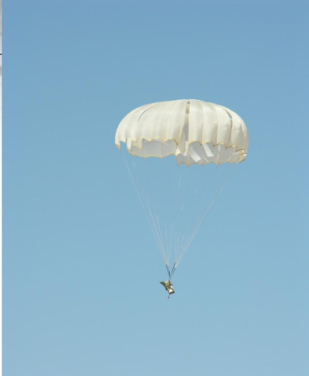
Extended Skirt Maltese Cross – late stage inflation
