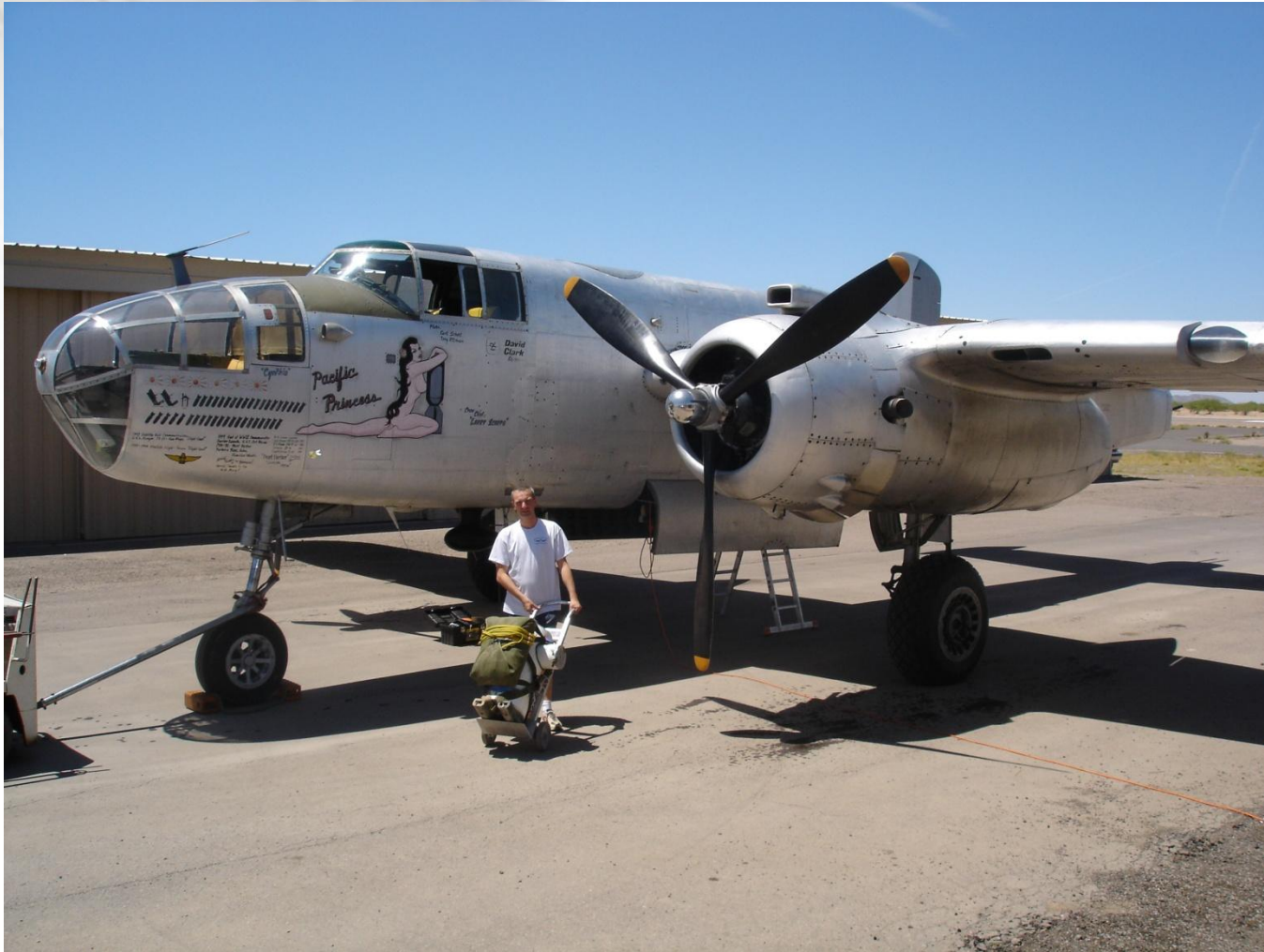
B25 "Pacific Princess" – Test Platform Instrumented Pipeman Test Dummy
